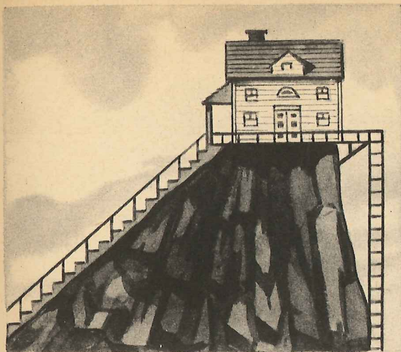
The stairway leading to the front door of the house on the left is longer than the straight ladder shown in the back of the house. Still, it takes less effort to climb the stairway. The winding road (right) is an inclined plane.
